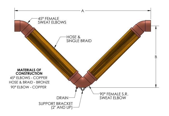
NOTE: V-LOOPS 2" AND LARGER INSTALLED IN ANY ORIENTATION OTHER THAN HANGING DOWN <u>MUST</u> HAVE THE 180° RETURN SUPPORTED. (SEE INSTALLATION INSTRUCTIONS.)
